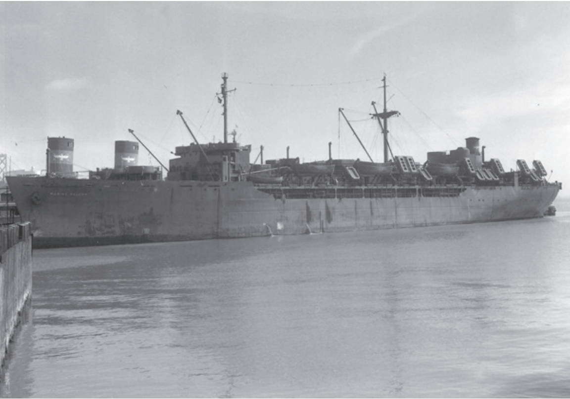
The Marine Falcon was a freighter ship with accommodations for 550 passengers.
