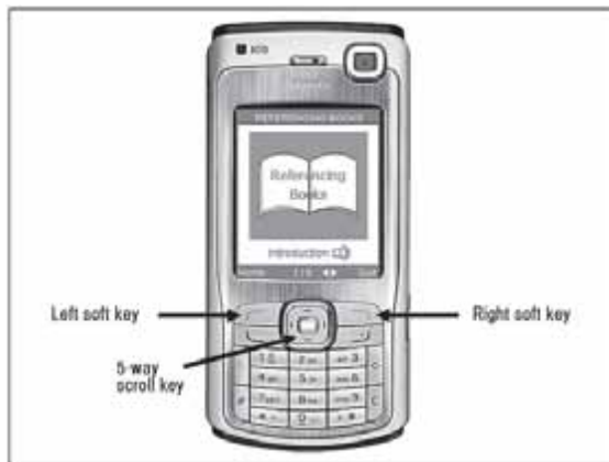
FIGURE 2 The Nokia N70 phone and keypad and the opening screen of Referencing Books
